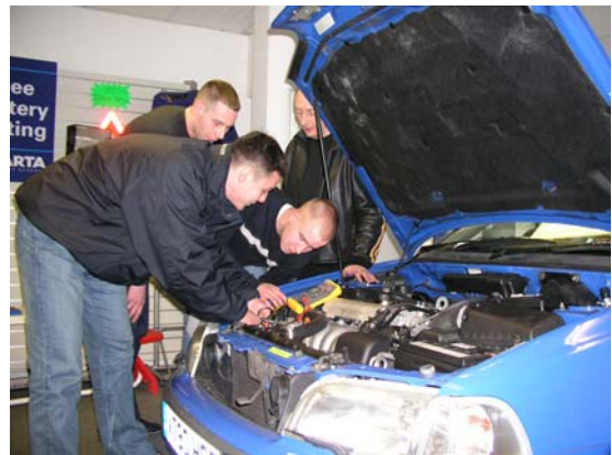
Delegates carry out circuit testing and analysis of digital multi meter test data
