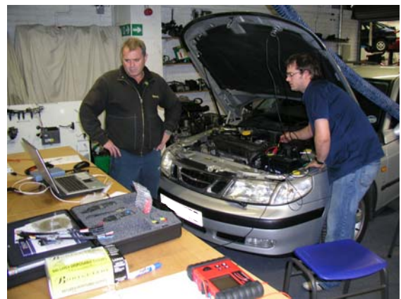
Testing sensors and actuators using PC based oscilloscope from Pico Technology
